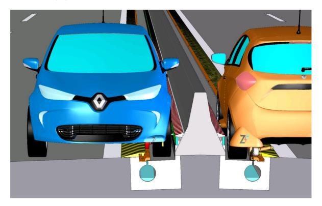
Ahead of the left front wheel a **multi-sensor device** continuously senses the lateral distance of the vehicle from the Jersey Wall and in **ZE-Drive** mode steers the car autonomously in all weather conditions to keep the left wheels at the center of the curbed track in a contactless fashion.
