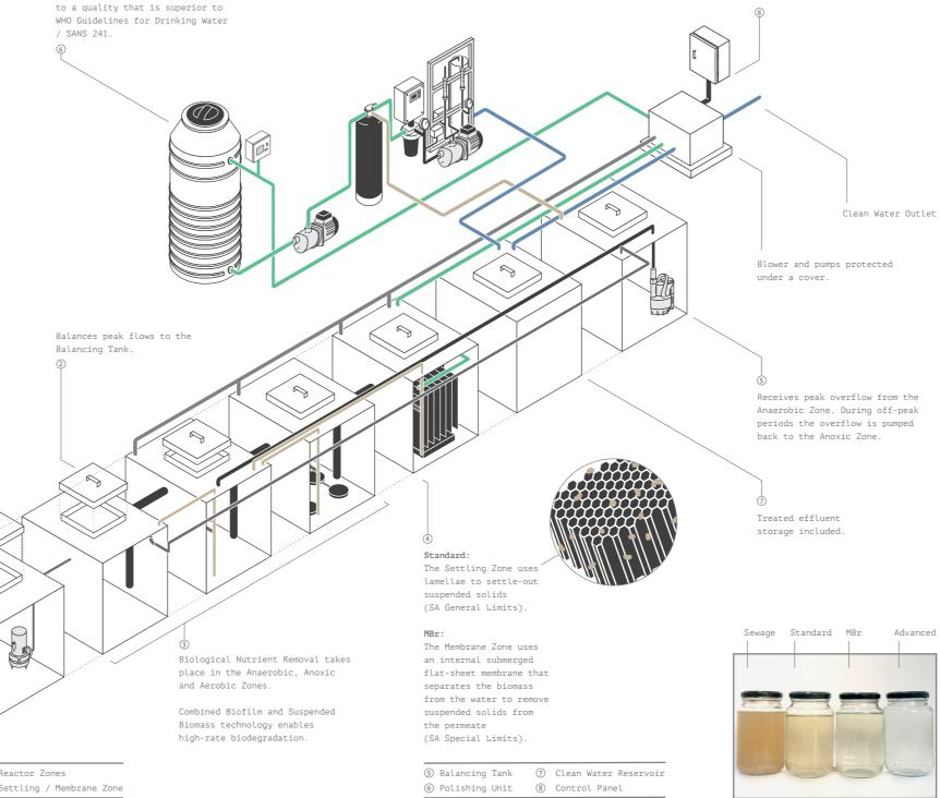
Sewage Pump Station ③ Reactor Zones (2) Anaerobic Zone ④ Settling / Membrane Zone Remote Monitoring VV with alarms. Clean Water Outlet
