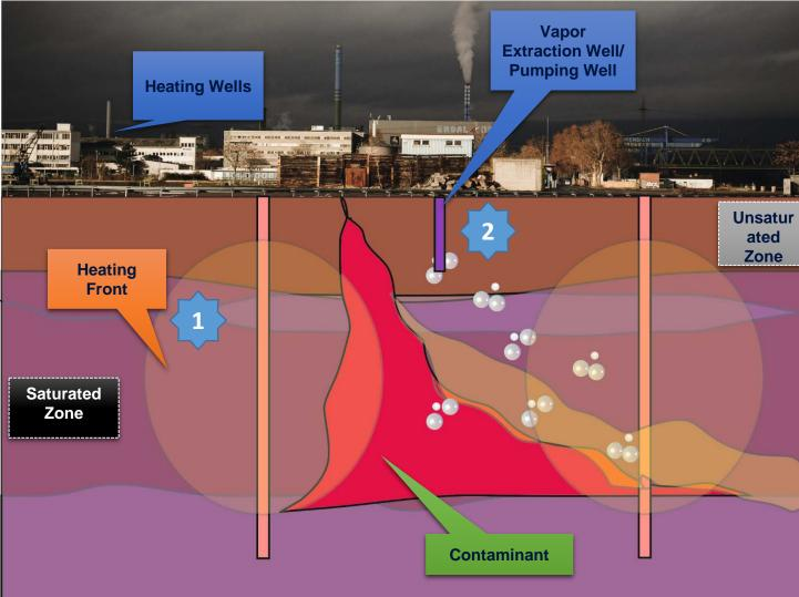
The contaminant mass in the soil is extracted by a soil vapor extraction equipment and the
