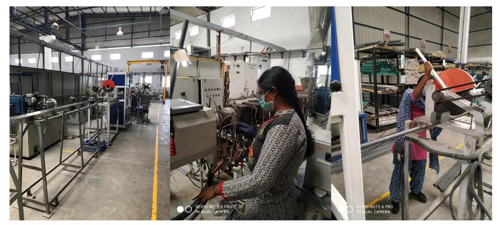
Converts recycled mixed plastics waste material into varied extruded sections such as rounds, hollow pipes, rectangular profiles with ~4x improved stiffness by reinforcing with natural fiber and glass fiber.
