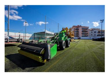
Rota Brush serves to **remove clean performance infill** (SBR, EPDM etc) for later reusing / reinstallation. Removal percentage (%) depends on circumstances like weather, evenness of infill, condition of artificial turf, type of turf, type of infill etc, in average 60% is removed in 1 day.
