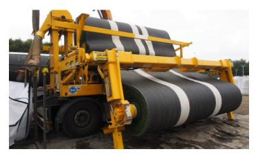
Separates the infill mixture (sand and rubber) from the artificial turf and stores the infill mixture in big bags. Uses CRAB for rolling up cleaned artificial turf.
