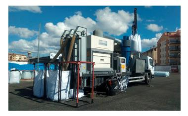
For drying, cleaning, sieving and separating the infill mixture to clean sand and rubber fractions stored in separate big bags. Separates also dust, old artificial turf fibres and other waste particles.
