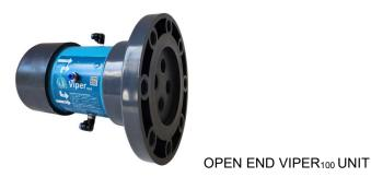
Weigh 3,54kg x 230mm-125mm dia x 320mm - max 6 Bar pressure - 50mm INLET connection.
