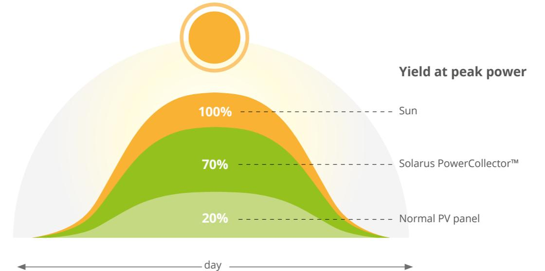
The use of the reflector, plus the use of concentrated solar power on the backside of the solar cells, combined with collected heat from the water/fluid cooling system of the receivers, ensures a yield which has been defined by the TÜV testing facility in Arizona as one of the highest they have ever measured.
