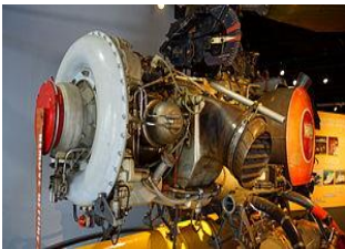
T50-BO-10 / 502-14) Manufactured for Boeing, this turboshaft has been a main line power plant for over 50 years
