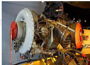
T50-BO-10 / 502-14) Manufactured for Boeing, this turboshaft has been a main line power plant for over 50 years
