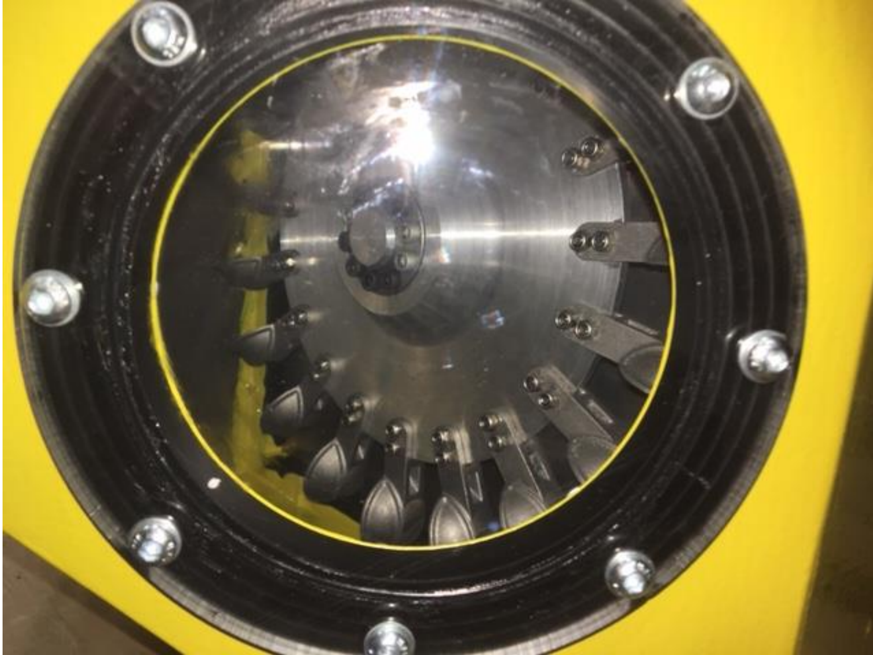
Turbine as seen through inspection hole
