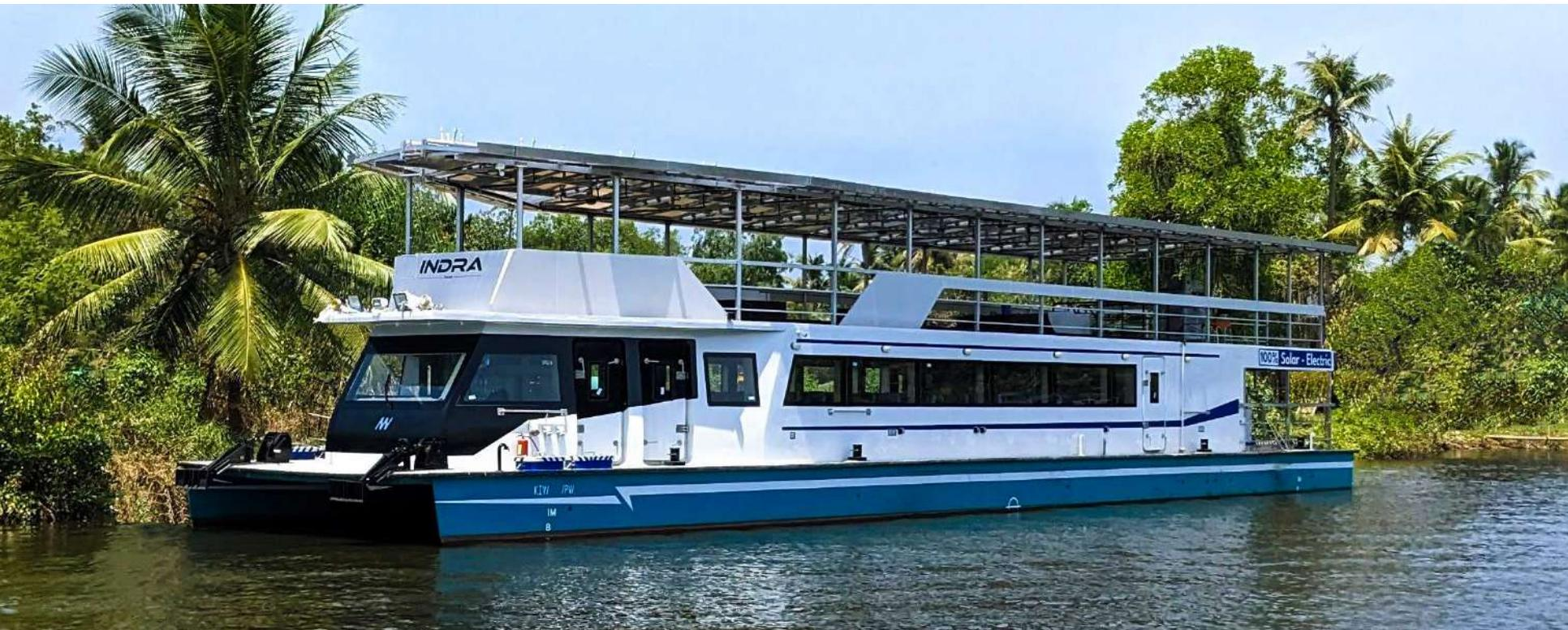
INDRA is a catamaran ferry boat with a GRP (Glass Reinforced Plastic, also known as FRP, or Fiber Reinforced Plastic) hull and an aluminium/FRP superstructure built under IR Class (Indian Register of Shipping, a member of the International Association of Classification Societies).
