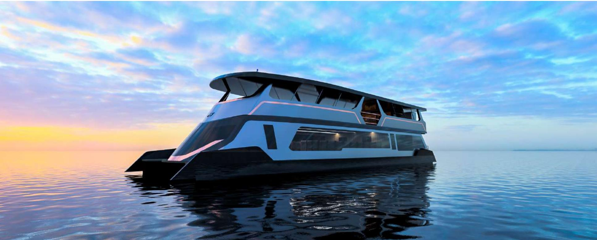
ZAYLE is a catamaran ferry boat with a GRP (Glass Reinforced Plastic, also known as FRP, or Fiber Reinforced Plastic) hull and an aluminum superstructure built under IR Class (Indian Register of Shipping, a member of the International Association of Classification Societies).
