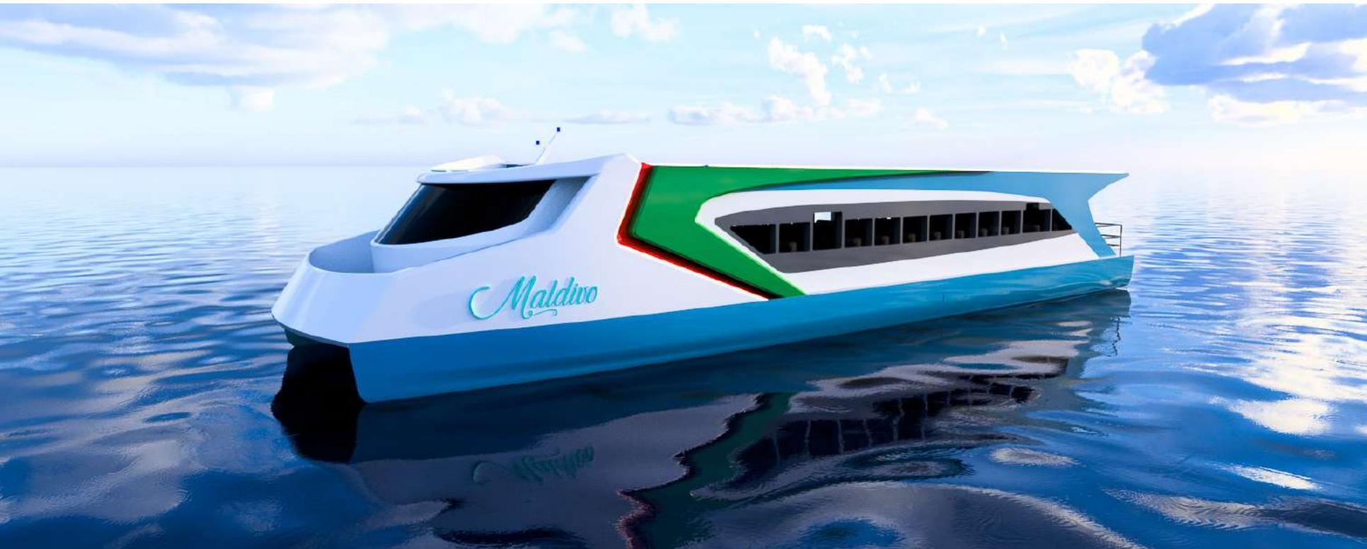
MALDIVO is a catamaran ferry boat with a GRP (Glass Reinforced Plastic, also known as FRP, or Fiber Reinforced Plastic) hull and an aluminium superstructure built under IR Class (Indian Register of Shipping, a member of the International Association of Classification Societies).
