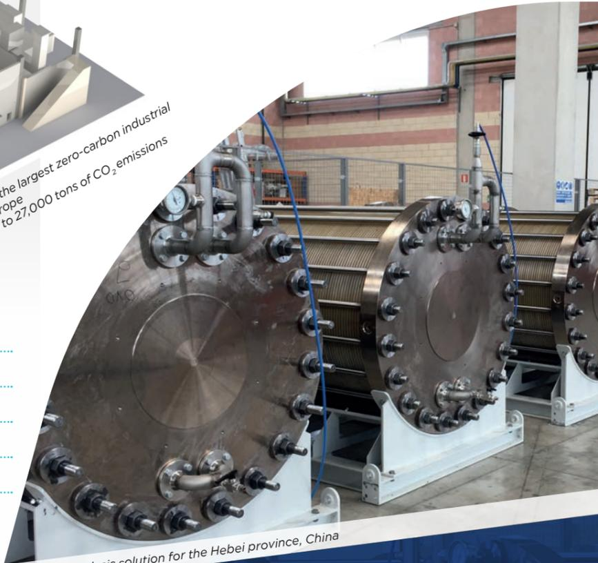
4 MW electrolysis solution for the Hebei province, China
