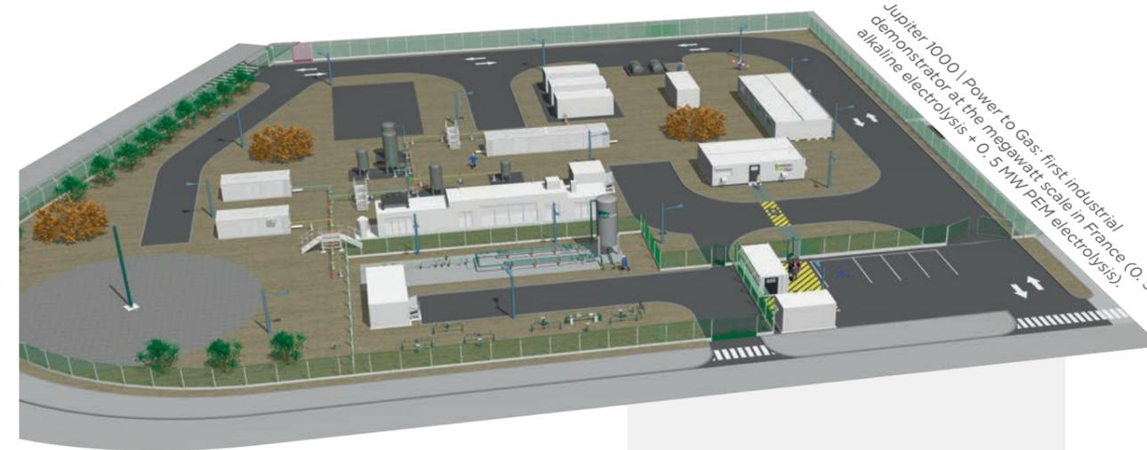
Jupiter 1000 | Power to Gas: first industrial demonstrator at the megawatt scale in France (0.5 MW alkaline electrolysis + 0.5 MW PEM electrolysis).
