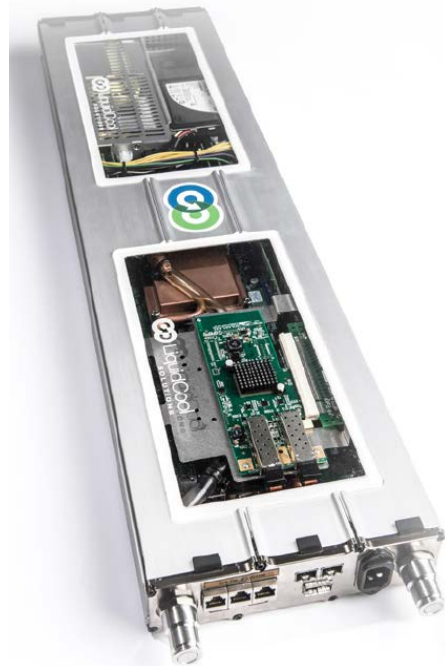
Figure ES-1. An LSS in liquid-tight aluminum housing Photo by Dennis Schroeder, NREL
