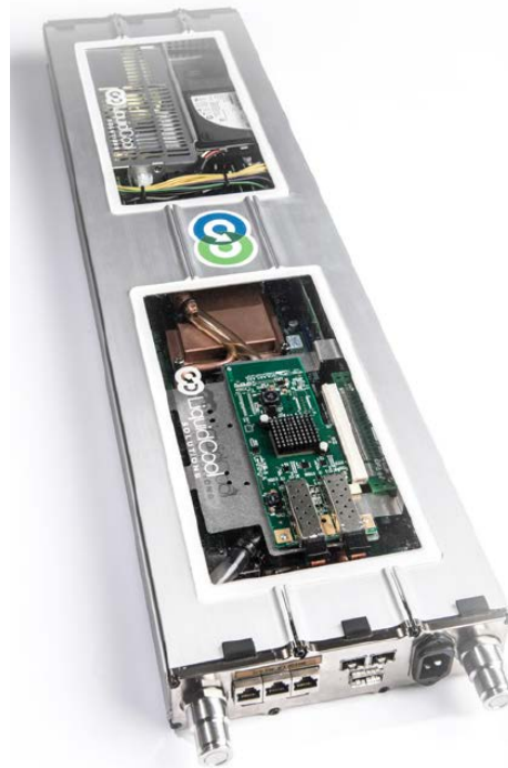
Figure 1. An LSS in liquid-tight aluminum housing Photo by Dennis Schroeder, National Renewable Energy Laboratory (NREL)
