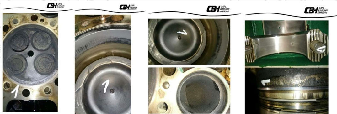
Cleaner Combustion → Less Soot → Cylinder Heads "Like New"
