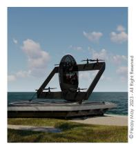
MTOW: 2200kg Take-off height: 5.15m Wingspan: 8m Footprint:
