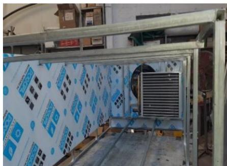
Inside the EZCond™ Module with 1 Heat Exchanger
