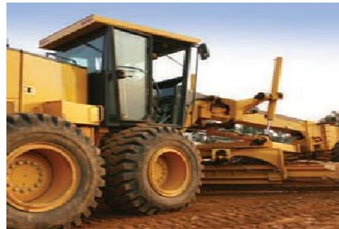
**3.** Mix applied ECORoads treated material in a windrow using a grader blade or soil mixer. Blade treated soil mix to create road level and crown surface.
