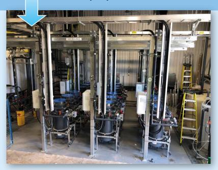
18 ECOTHOR-16R Reactors configured to operate in electrocoagulation mode with ANO1M (Al Alloy) & ANO2M (Mg alloy) anodes.
