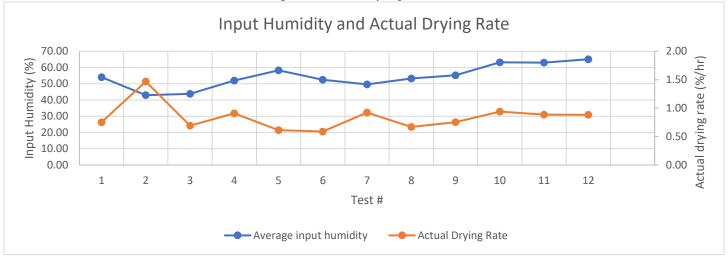
There is an inverse relationship between input humidity and the drying rate. Higher humidity has slightly adverse effects on the drying rate, mostly due to the input air's ability to carry the released moisture from the bed. Higher CFM will likely solve this.
