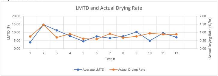
There is no real relationship between the log mean temperature difference and the actual drying rate, though it does trend proportionally. This means that the temperature difference from inlet to outlet has no bearing on the drying rate.
