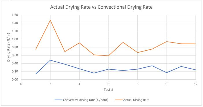
Below is a chart of the data above. The far right column shows the multiplier effect the RF has on the drying rate across various tests.
