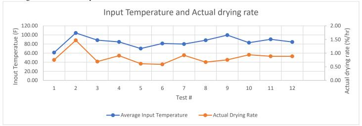
There is a somewhat proportional relationship between input temperature and drying rate. Higher temperature air has a higher moisture carrying capacity, so the drying rate is generally increased when the ambient temperature is hotter.
