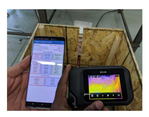
Material Temperature = 67.8° F Exit Air Temp = 5° F > Ambient Humidity = 46% above Ambient!!
