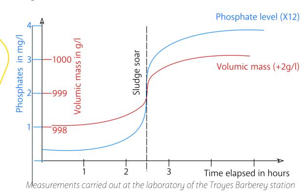
The intracellular content is then diluted in the settling medium, which gives a sudden density surge to 2g/l in the test cylinder. There is an inversion of thrust on the bacterial envelope that has been emptied of its contents. That is the phenomenon behind the soaring sludge.
