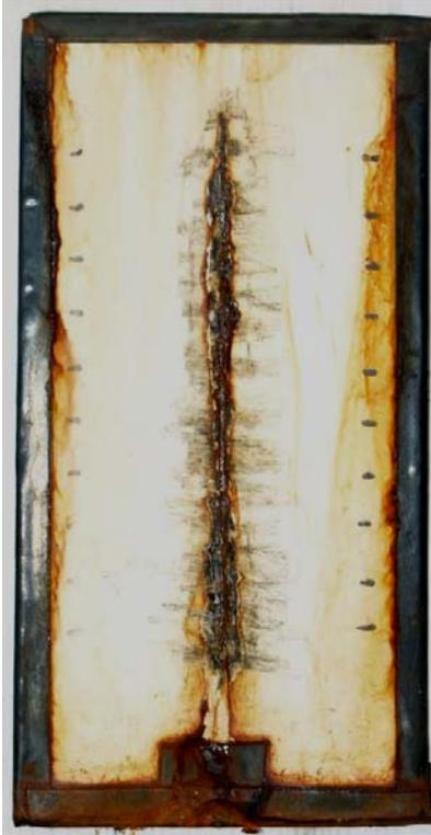
**Panel II-91-6 – 9404 Hours Salt Fog Exposure (Scraped at 8372 Hours)**
