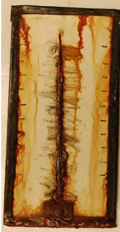
**Panel II-91-10 – 11420 Hours Salt Fog Exposure (Scraped at 8372 Hours)**
