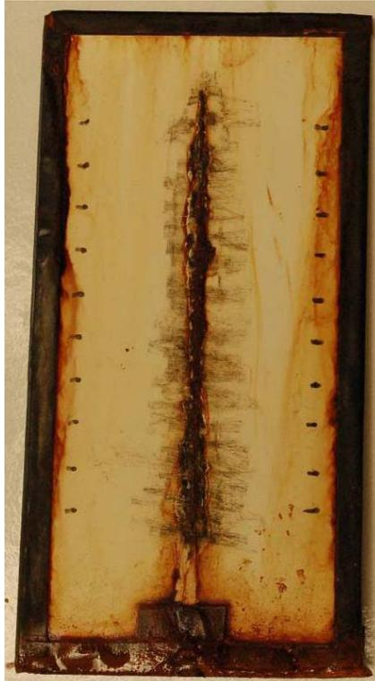
**Panel II-91-6 – 11420 Hours Salt Fog Exposure (Scraped at 8372 Hours)**
