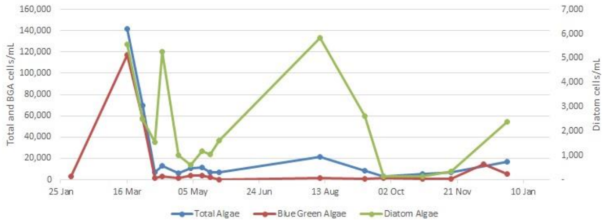
Figure 2 – Dam 2 – Raw water storage treated with Diatomix to reduce BGA cell counts.
