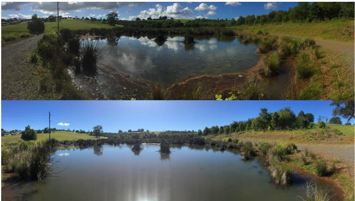
Figure 13 – The release point of the wetland cell (Cell 3) that is fed Cells 1 and 2. Cell 1 was the untreated Control cell and Cell 2 was also treated with Diatomix . The top picture is Day 0 of treatment and the bottom picture is 100 days later.
