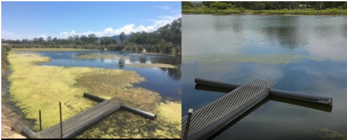
Figure 7 - Case Study 4 - Weed growth in a Barramundi farm water storage lagoon. Normally the lagoon required mechanical harvesting every 5 weeks. With Diatomix dosing, the photo on the right was taken 22 weeks after Diatomix dosing.
